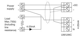
2 wires system : DC power supply with Analogue output Power + supply - Load Max.750Ω (Including line resistance) - UW/UWC
