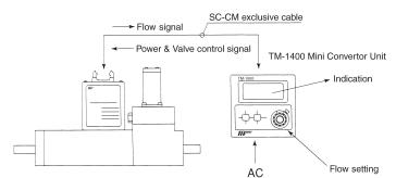
TC-3100 MINI THERMAL MASS FLOW CONTROLLER TC-3300/3600/3800 MINI THERMAL MASS FLOW CONTROLLER
