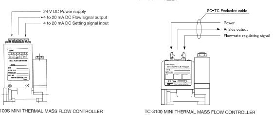
TC-3100S MINI THERMAL MASS FLOW CONTROLLER
