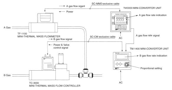
This is an example of mixing of A and B gas in a given proportion. The flow rate of A gas is measured by TF-1000 series Mini-Thermal Mass flowmeter and its signal is input to TM-1400 as External setting signal. At TM-1400 Converter, freely adjustable setting dial is provided for set gas proportion and TM-1400 sends valve signal to TC-3000 Mini-Thermal Massflow Controller to control the operation of control valve.
