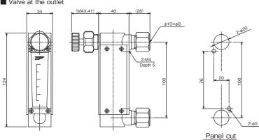
Note: Use non-magnetic material for the panel when the alarm output code is one of A to D.
