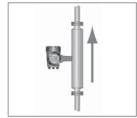
②When installing the flowmeter on the vertical line, install it in upward flow direction.
