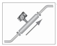
③When installing the flowmeter on the slant line with upward flow, place the converter or the terminal box of remote type above the measuring tube.
