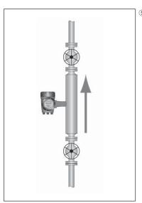
When installing the flowmeter on the vertical line, provide with stop valves at both upstream and downstream to keep the flowmeter to be filled with liquids, which is necessary to perform zero adjustment.
