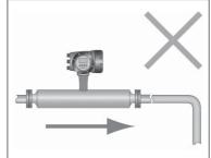
(4) When installing the flowmeter on the horizontal line, make the upstream and downstream pipings be filled with liquids. Do not bend these pipings downward at the vicinity of flowmeter. To avoid unnecessary accumulation of gasses, do not install the flowmeter on the upper part of associated pipings in such processes containing air or gas.
