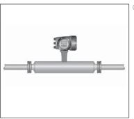
①When installing the flowmeter on the horizontal line, place the converter or the terminal box of remote type above the measuring tube.
