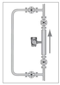
(®) It is highly recommended to equip with bypass and stop valves for maintenance purpose.
