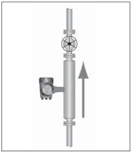
①Install a control valve downstream if required to avoid the cavitations caused by throttling of valve.
