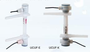
A PFA ultrasonic flow meter designed for high-precision measurement of small-flow ultra-pure water and various chemicals. The wetted parts are all made of PFA, and there are no moving parts, no mechanical seal parts such as O-rings that easily cause liquid pooling, and an ideal clean structure.
