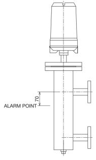
70mm below the center line of upper nozzle both for side~side and side~bottom type chambers.
