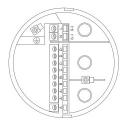
Protection cover is provided for power supply terminals.
