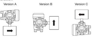
The mounting position will be arranged according to the customer's request when ordering.
