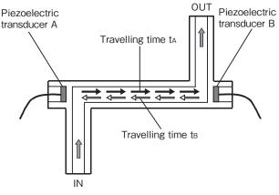
Figure 1 Operating principle
