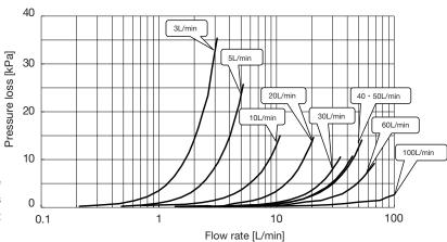
Note:This graph shows reference values for pressure losses that may occur when there are no drifts or swirling flows and the viscosity is equivalent to that of water.
