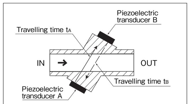
Figure 1 Operating principle
