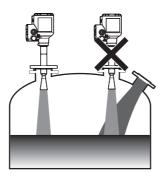
• For tanks whose bottom is not flat but dish- or cone-shaped, the measuring range is from the lower end of the dead zone to the lower end of the cylindrical part of the tank. It is not possible to measure the level precisely below the cylindrical part.
