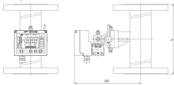
This outline dimension is for the liquid measurement. An indicator is fixed at the top of isolation valve in case of gas measurement.
