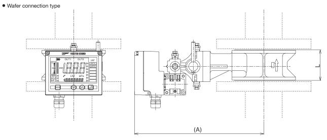
This outline dimension is for the liquid measurement. An indicator is fixed at the top pf isolation valve in case of gas measurement.
