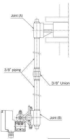
This outline dimension is for the liquid measurement. An indicator is fixed at the top of isolation valve in case of gas measurement
