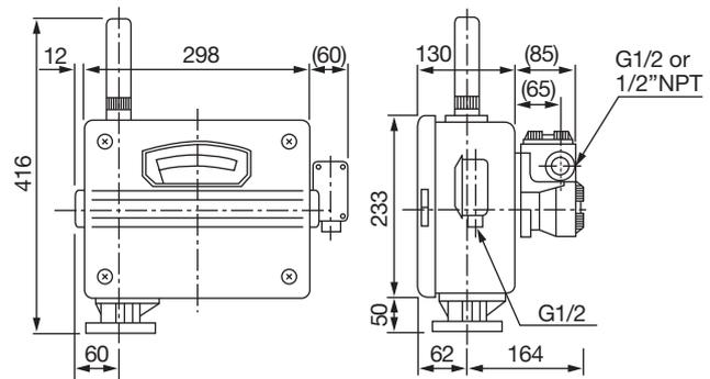
Fig. 15 : Indicator and transmitter assembly (FS-517W)
