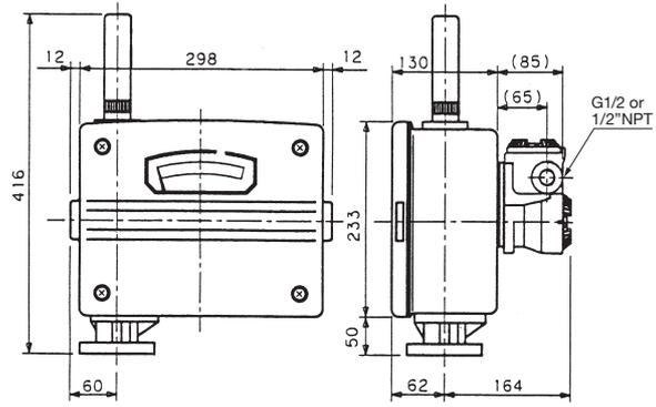
Fig. 13 : Indicator and transmitter assembly (FS-512W and FS-512E)
