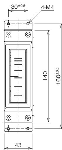
Note: Metal fixtures should not be used for supporting the flowmeter.
