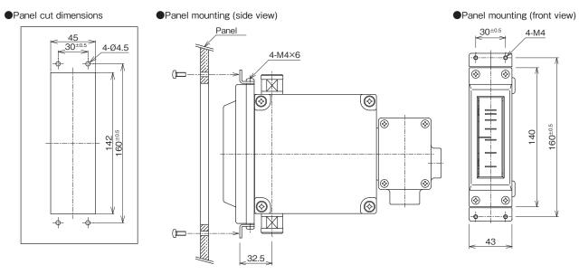
Note: Metal fixtures should not be used for supporting the flowmeter.
