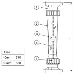
Above figure is for SUS316 float with float rod version. No float rod is provided for other float material versions.
