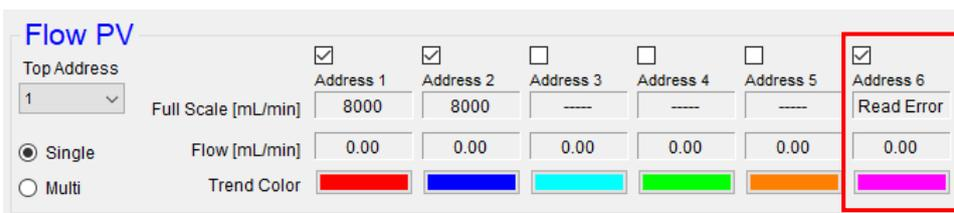
The 'Flow PV' window is shown with 'Address 6' selected. The 'Full Scale' for Address 6 is 'Read Error' and the 'Flow' is '0.00'. The 'Trend Color' for Address 6 is highlighted with a red box.
