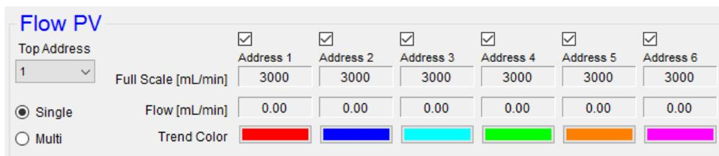
The 'Flow PV' window shows 'Top Address' set to 1. It has six columns for 'Address 1' through 'Address 6'. Each column has a checked checkbox, a 'Full Scale [mL/min]' field (3000), a 'Flow [mL/min]' field (0.00), and a 'Trend Color' field with a color swatch.
